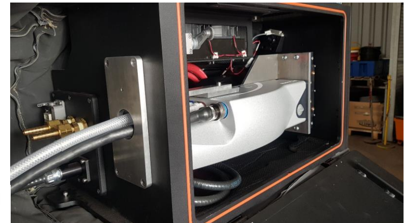
LUS-measurement head with water cooling
